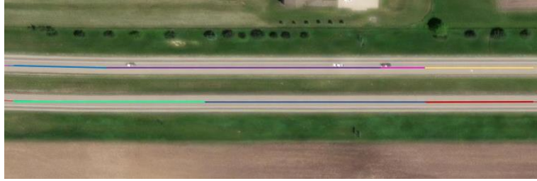
Figure 5.16. Colored lines representing the reference line on a divided highway, which was used for the DFRL calculation
