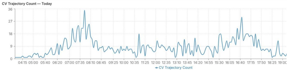
Figure 4.11. CV trajectory counts over the day for work zone 1EA – Mainline WB 1
