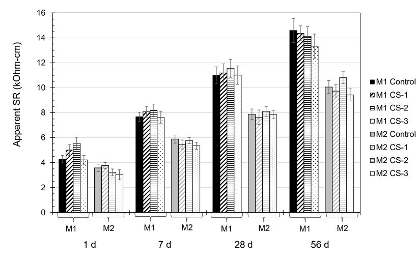
The apparent SR is not significantly different for the control samples without CS compared to those with CS after very early ages.
