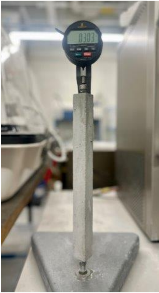
Mortar bar method per ASTM C1260 (Alkali reactivity of aggregates)
