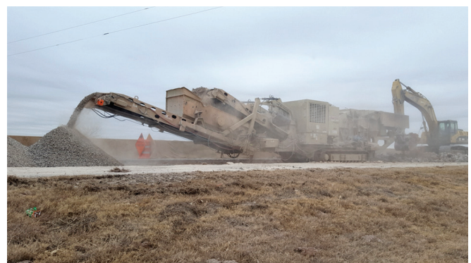
Figure 2. Mobile on-grade production of RCA
