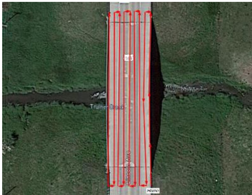
Figure 46. Manual mission flight at 15 ft (4.6 m) AGL
