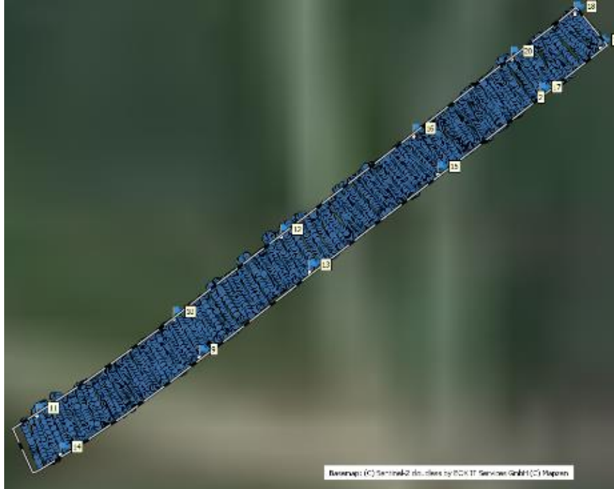
Figure 16. sUAS image points and GCPs represented using white boxes
