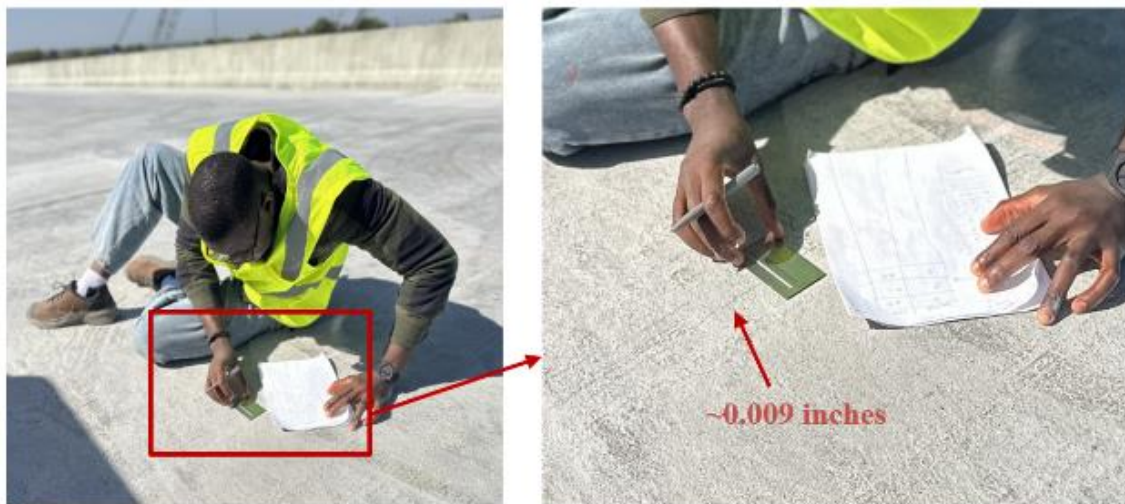
Figure 15. Ongoing measurement of observed hairline cracks
