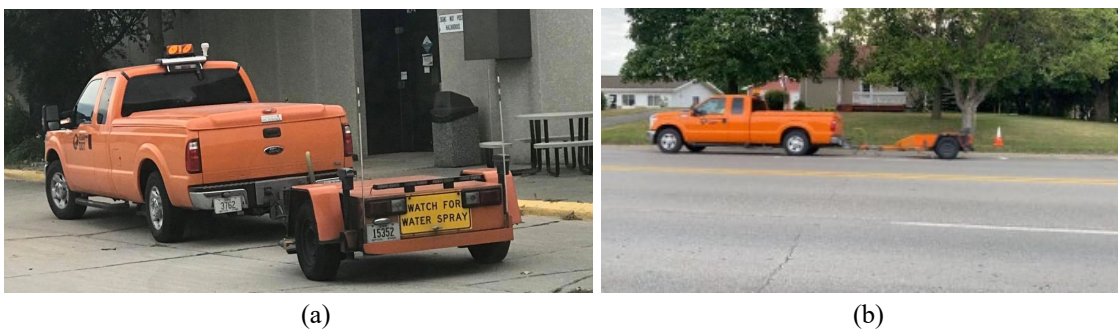
Figure 19. Locked-wheel skid tester: (a) close-up view and (b) in operation
