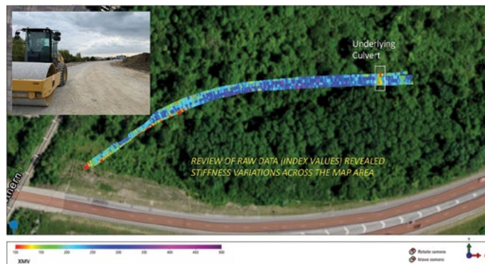
Figure 16. I-465/I-69 stabilized pavement foundation showing stiff conditions
