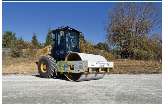
(c) Caterpillar CS56 vibratory smooth drum roller outfitted with mapping hardware kit
