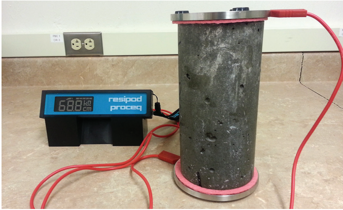
Figure 3. AASHTO TP 119 bulk resistivity test
