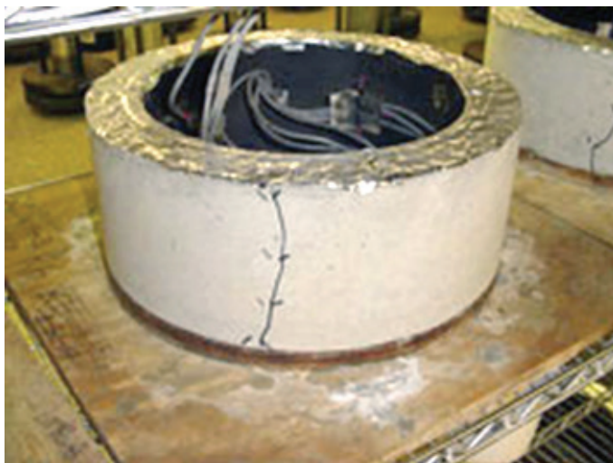
University of North Carolina at Charlotte, used with permission Figure 1. AASHTO T 334 cracking tendency test
