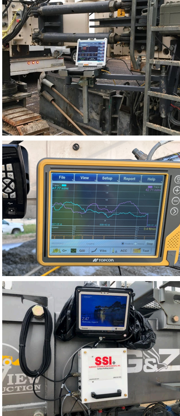
Figure 3. Various RTS displays: Ames RTP laptop (top), GSI tablet (middle), SSI OPP tablet (bottom)
