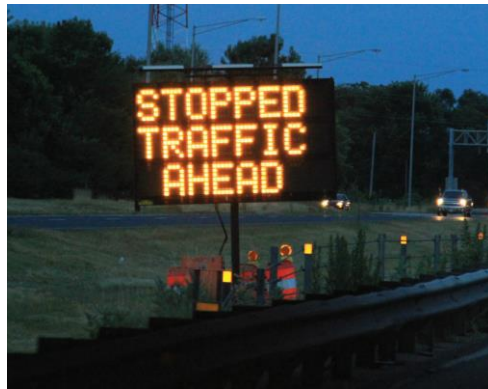
Figure ES1. Example queue warning display on portable CMS
