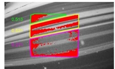
Snow coverage detection in daytime images: original optical and infrared images (left) and segmentation based on optical (middle) and infrared (right) images
