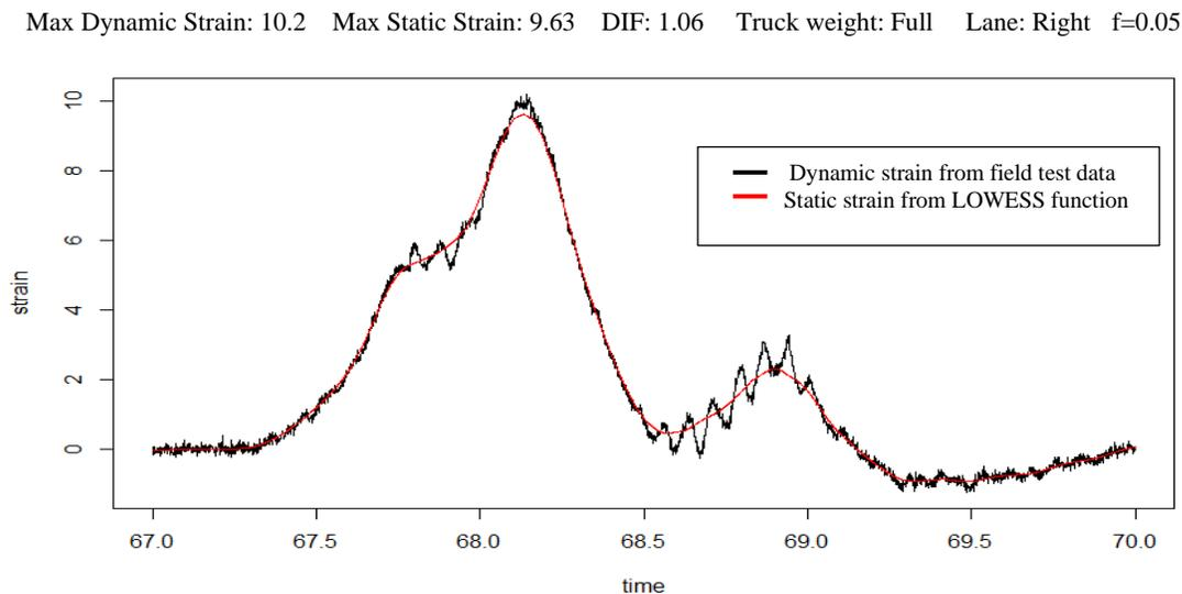
**Figure 1. Data from vehicle 1 on bridge 4050.0S017**
