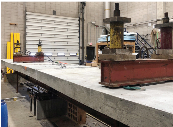
Laboratory testing setup for full-scale link slab
