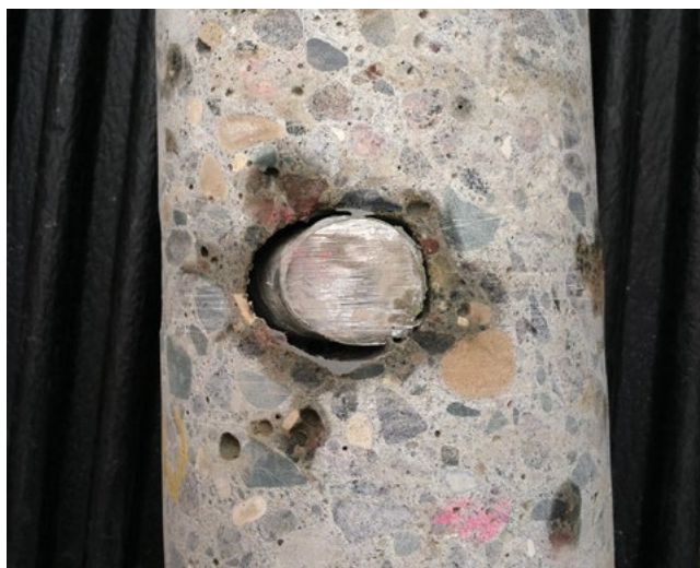
Figure 6.19. Socketing around dowel bar on core taken from FDR
