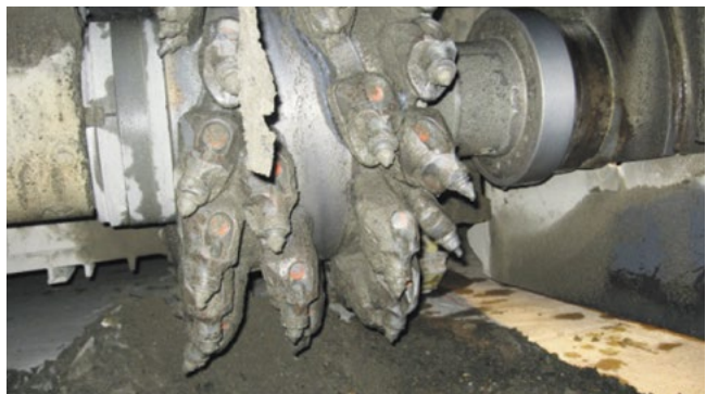
Figure 5.15. Rock saw capable of producing rounded milling (top) and milling pattern (bottom)
