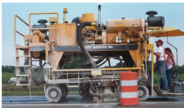
Figure 8.8. Diamond-bladed slot-cutting machine
