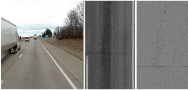
Figure 3.3. Typical images from a 3D data collection van showing a cross-stitched longitudinal crack and the right-of-way (left), the range in the vertical direction (center), and the downward-facing camera view (right)
