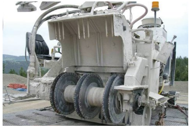
Figure 8.10. Equipment capable of cutting three dowel bar slots at once
