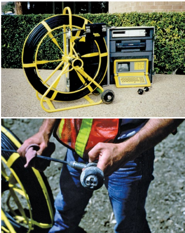
Figure 7.23. Video system (left) and camera head (right) for drainage system inspection
