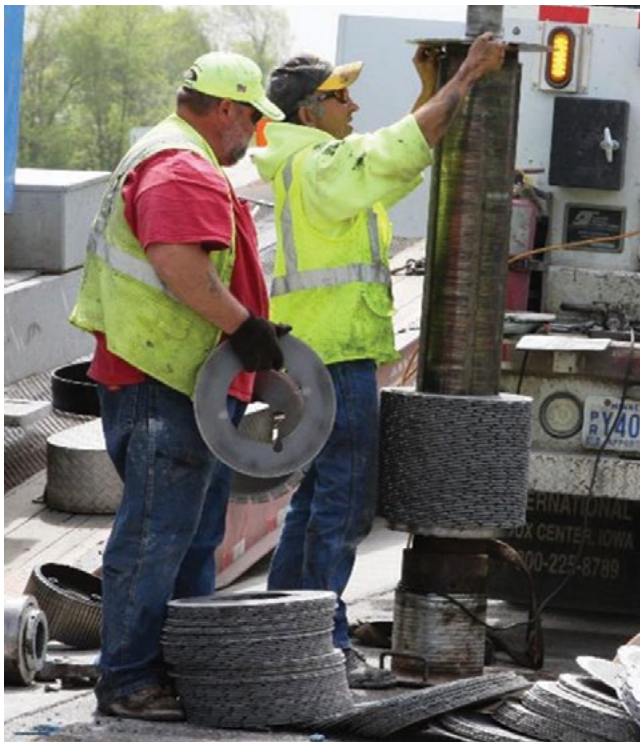
Figure 9.8. Stacking spacers and blades on a diamond grinding machine's cutting head
