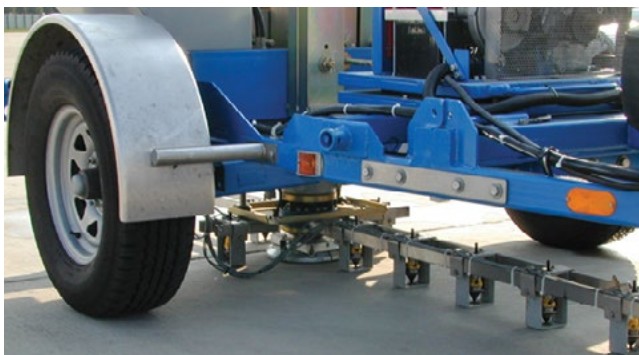
Figure 3.7. FWD showing load plate and sensor bar for joint testing
