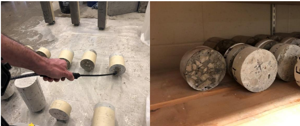
Figure 1. Application of sealer (left) and curing specimens vertically (right)
