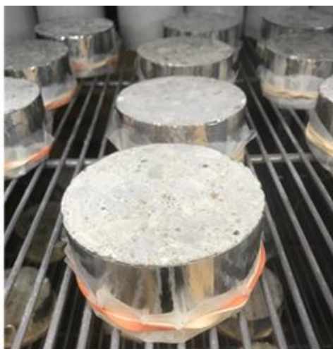
Figure 2. Desaturation of specimens in environmental chamber
