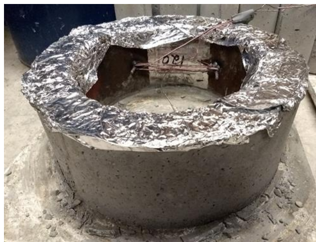
Figure 4. Concrete ring undergoing restrained shrinkage
