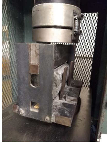
Figure 5. Concrete cylinder and bearing device loaded into the testing machine
