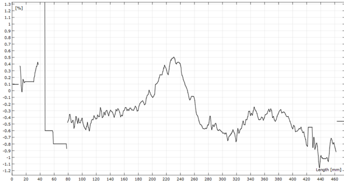
Figure 14. Final tensile strain chart for Specimen 0K
