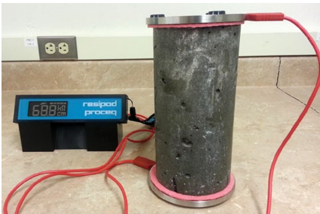
Figure 4.3. AASHTO TP 119 bulk resistivity test
