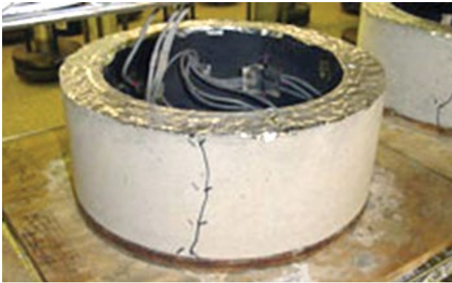
Figure 4.1. AASHTO T 334 cracking tendency test
