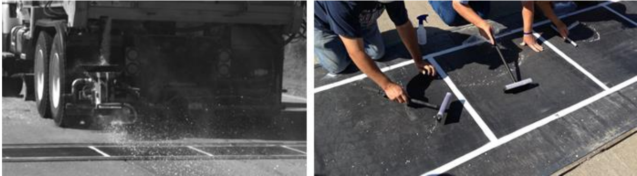
Figure 3. Salt sample collection per run and grid square
