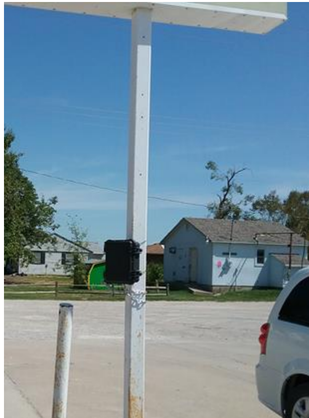
Figure 4-7. Jamar radar data collection unit
