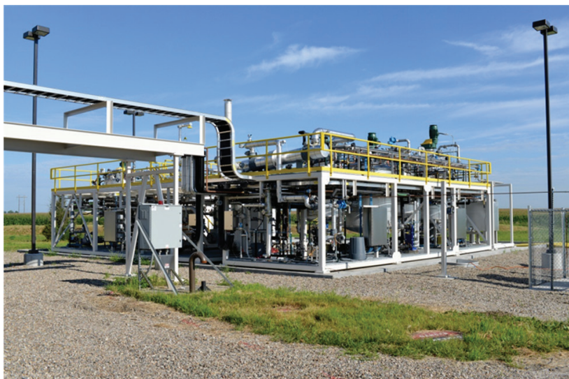
Biopolymer pilot plant capable of producing 10 tons of polymer per week that was built just west of Iowa State University at its BioCentury Research Farm as part of this research project
