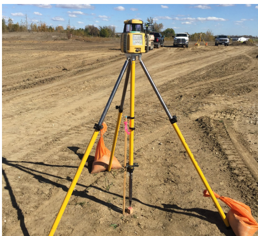
Figure 10. A rotating laser on a control point. Photo courtesy: Snyder & Associates, Inc.
