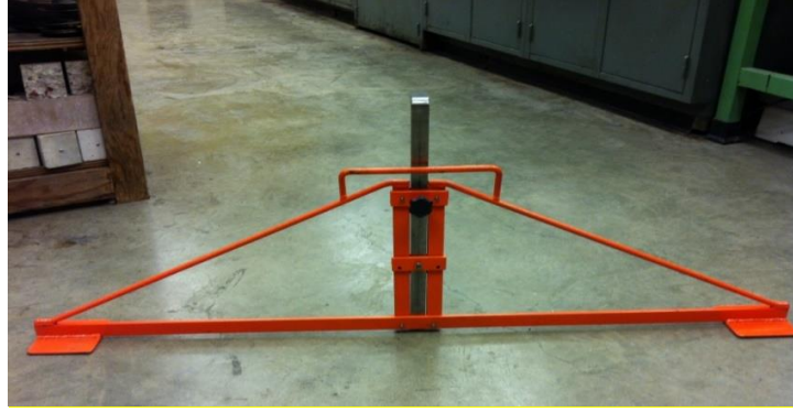
Figure 1. Deflectometer for measuring rutting
