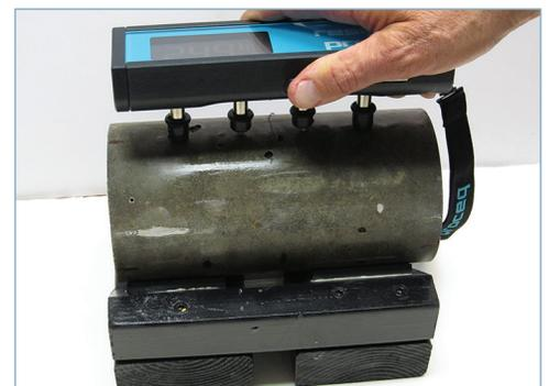
Cylinder sample testing with surface resistivity meter
