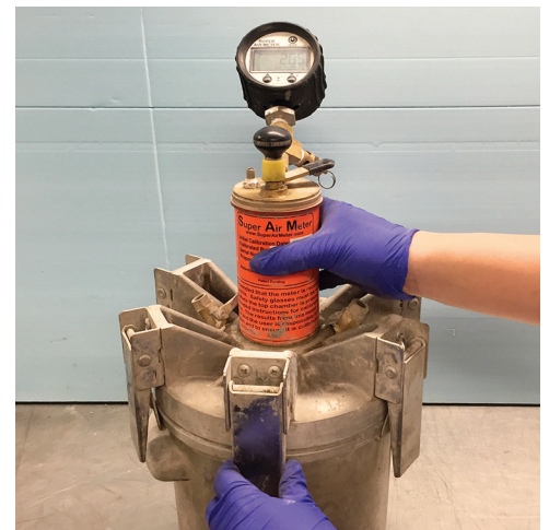
Super air meter indicates air distribution in concrete for freeze-thaw durability
