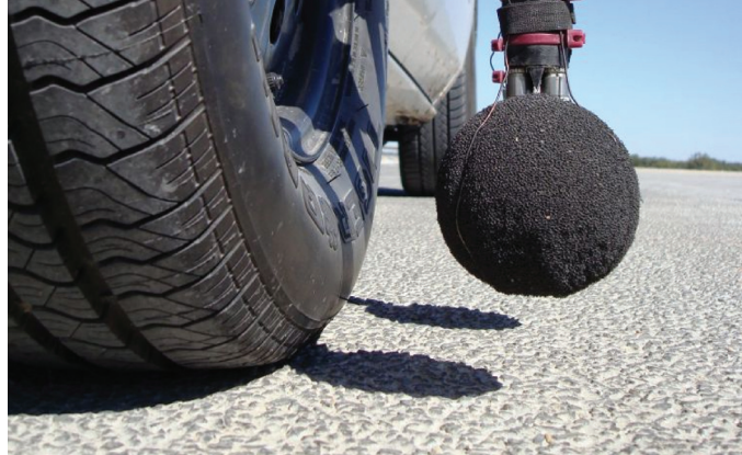
Figure 6. OBSI for measuring tire-pavement noise at the source
