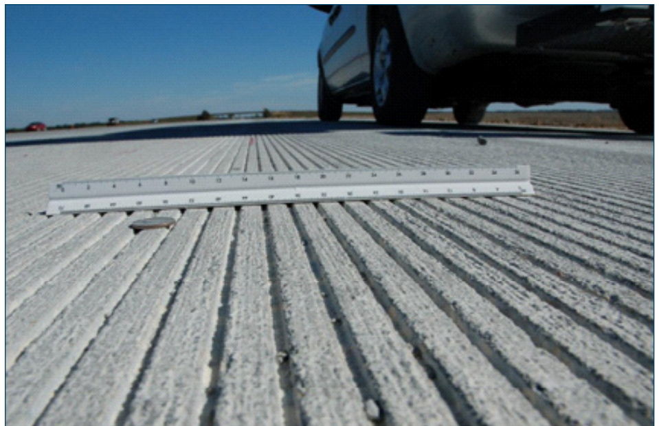
Longitudinal grooving and turf drag test section from the Concrete Pavement Surface Characteristics Program
