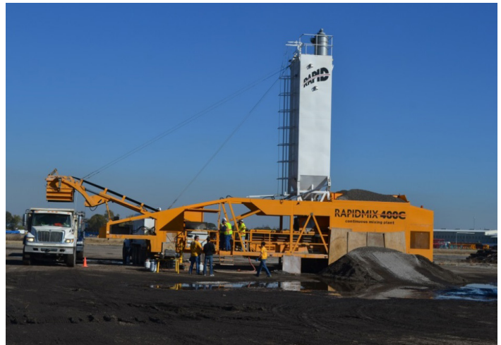
Figure 6. Twin shaft pugmill
