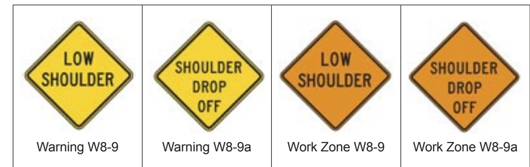
Figure 2-1. MUTCD warning signs for edge drop-off
