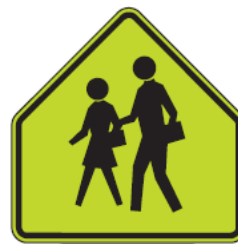
School advance crossing sign
