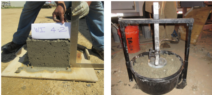
Figure 4. Box Test (left) and V-Kelly test (right) for evaluating workability of the concrete mixture
