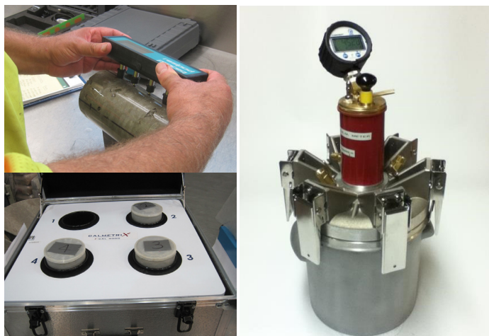
Figure 1. Surface resistivity test (top left), calorimetry test (bottom left), Super Air Meter (SAM, right)
