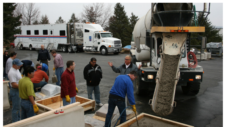
Figure 5. Photo of FHWA's Mobile Concrete Trailer providing hands-on technical training on PEM testing procedures
