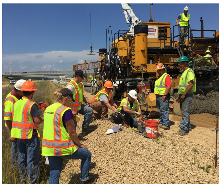
Figure 3. Contractors and state highway agency personnel measuring air content using the SAM
