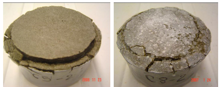
Figure 6. Expansion in Mortar Specimens Soaked in (a) 17% \text{CaCl}_2 and (b) 15% \text{MgCl}_2 for 150 days at 40°F Note: specimens were never frozen (Source: South Dakota Department of Transportation)
