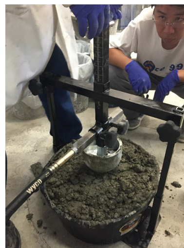
Figure 13. Ongoing V-Kelly test
