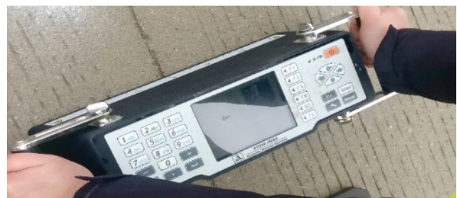
Figure 2. MIRA ultrasonic shear-wave tomography device being used to collect joint activation data
