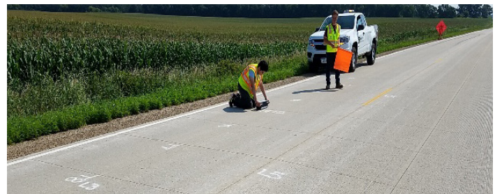
Figure 1. Joint activation data collected on an existing overlay in Worth County, Iowa using a MIRA device placed over saw cuts
