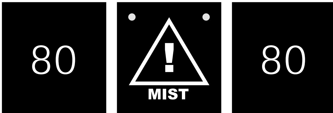
Figure 6. Representation of Matrix Signs of a Fog Warning System in the Netherlands.
