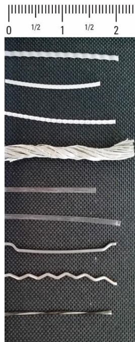
Figure 3.1. Examples of different macrofiber types, top to bottom: crimped, embossed, bi-tapered, and twisted synthetic; straight fibrillated synthetic (two images); hooked-end and crimped steel; and twisted basalt
