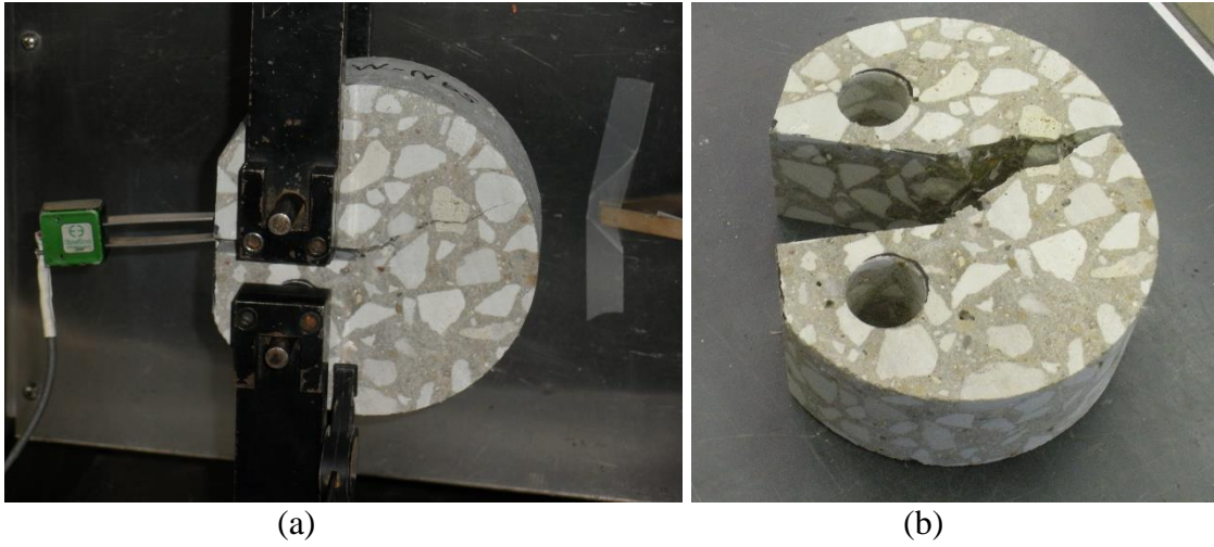
Figure 7.12. Fracture geometry of the DCT test for FRC (a) during and (b) after testing
