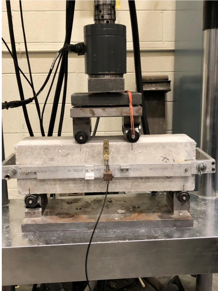
Figure 7.2. ASTM C1609 test setup showing the LVDT measuring the deflection at the top of the beam at midspan and the ASTM C1812 roller assembly
