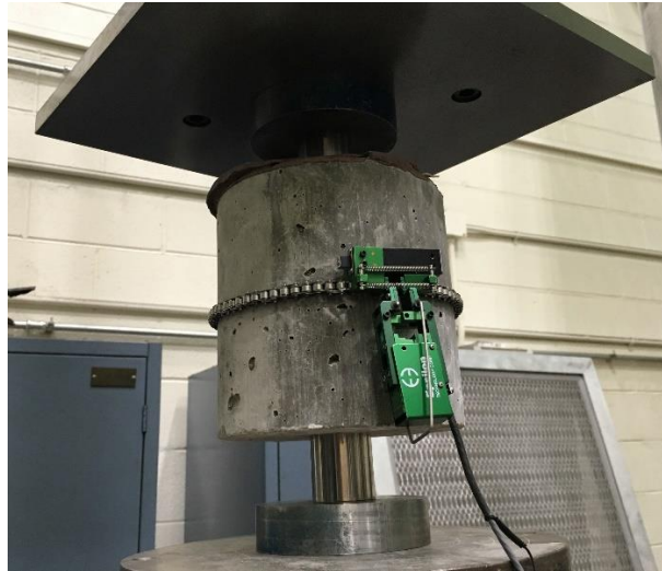
Figure 7.9. Barcelona test (double-punch test) setup with a circumferential extensometer attached at the mid-height of the FRC cylinder to measure TCOD
