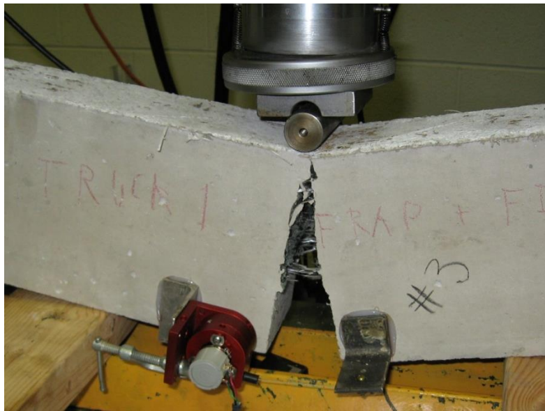
Figure 4.1. Example of the post-cracking behavior of notched FRC beam specimen with synthetic macrofiber volume of 0.43%
