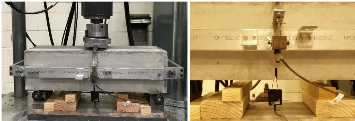
Figure 7.7. EN 14651 setup, with an LVDT measuring deflection at the beam mid-span (left) and a clip-on gauge measuring CMOD (right)
