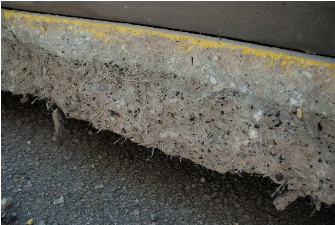
Figure 2.2. Two-lift concrete slab with a 2 in. plain concrete top lift and a 4 in. bottom lift containing reclaimed asphalt pavement aggregates and 0.43% synthetic macrofibers by volume
