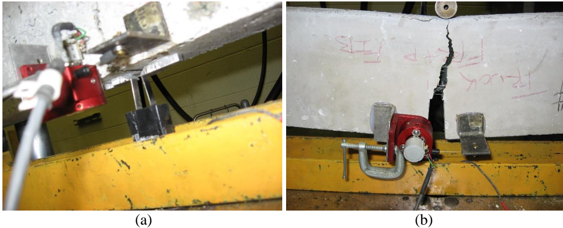
Figure 7.10. Notched beam fracture testing of FRC showing (a) the clip-on gauge attached to knife edges on the bottom of the beam across the notch, (a, b) the string potentiometer attached to the exterior of the beam, and (b) the fractured specimen
