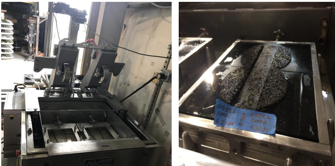
Figure 3-9. Hamburg wheel tracking device: test device, left, and mixtures after test, right
