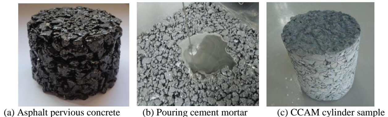
Figure 1.1. Casting cement asphalt mixture (CCAM)
