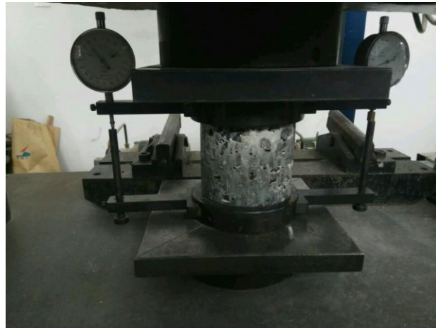
Figure 4.7. Resilient modulus test
