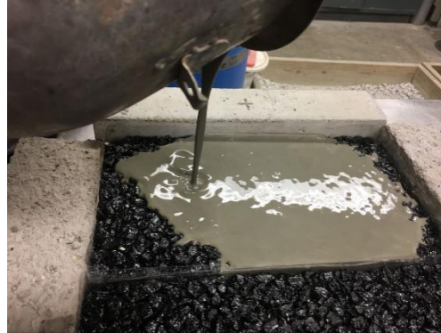
(b) Pouring grouting materials
