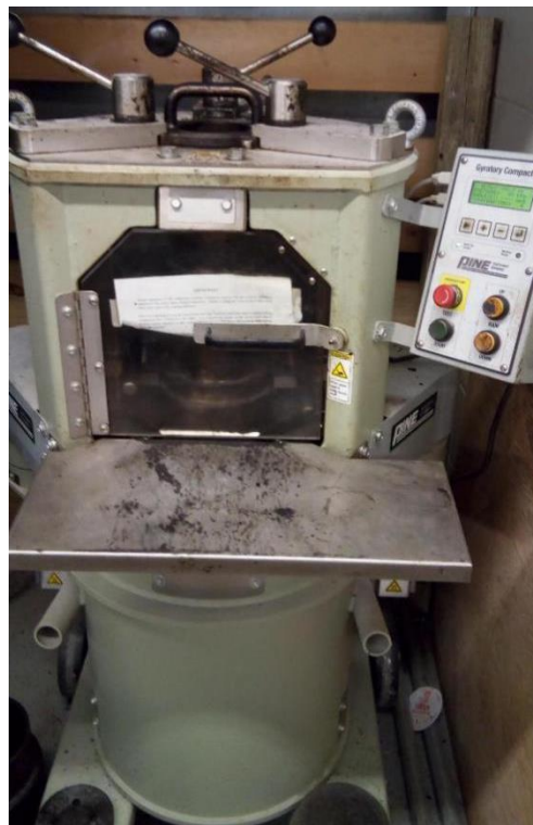
Figure 3.2. Gyration compaction meter
