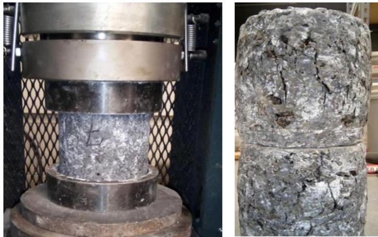
Figure 4.2. Compressive strength test and failed samples
