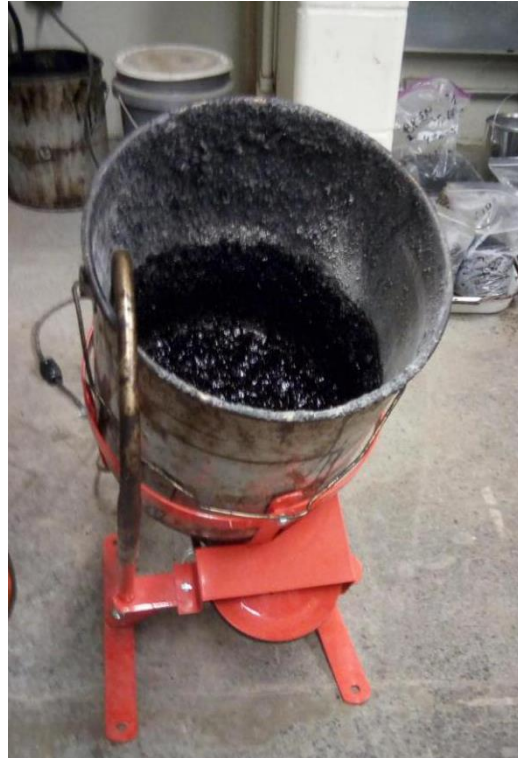
Figure 3.1. Mixer of asphalt mixture
