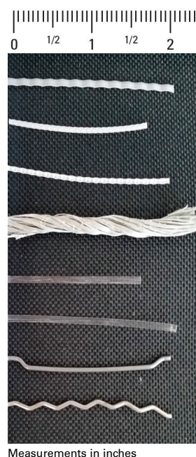
Figure 5. Examples of different macrofibers, top to bottom: crimped, embossed, and bi-tapered synthetic; twisted synthetic; straight fibrillated synthetic (two images); and hooked end and crimped steel
