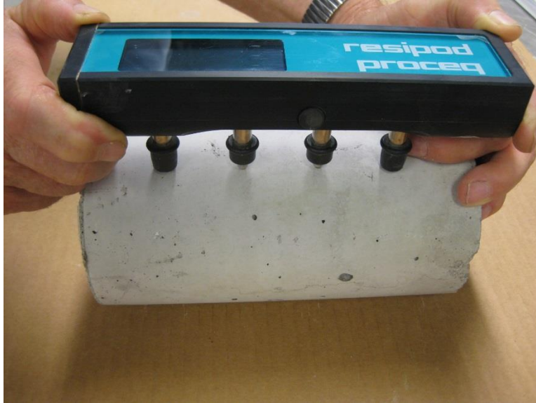
Figure 13. Resistivity measurement device
