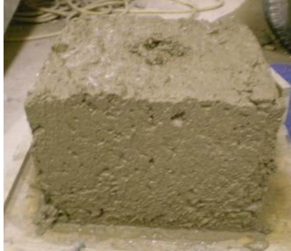
Figure 20. Box test sample after removing the forms
