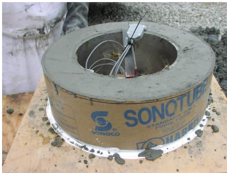
Figure 15. A ring shrinkage specimen
