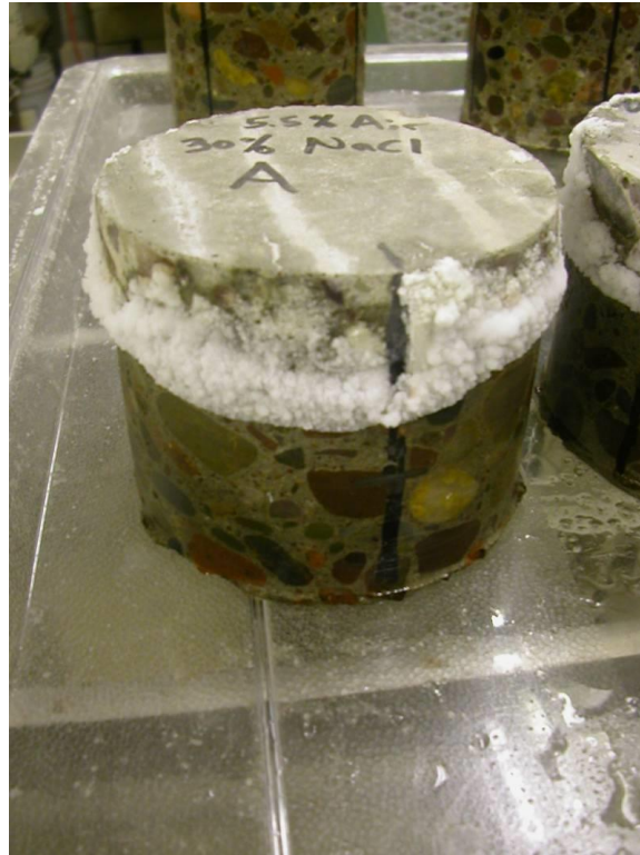
Figure 7. Salts wicked up a partially-immersed sample
