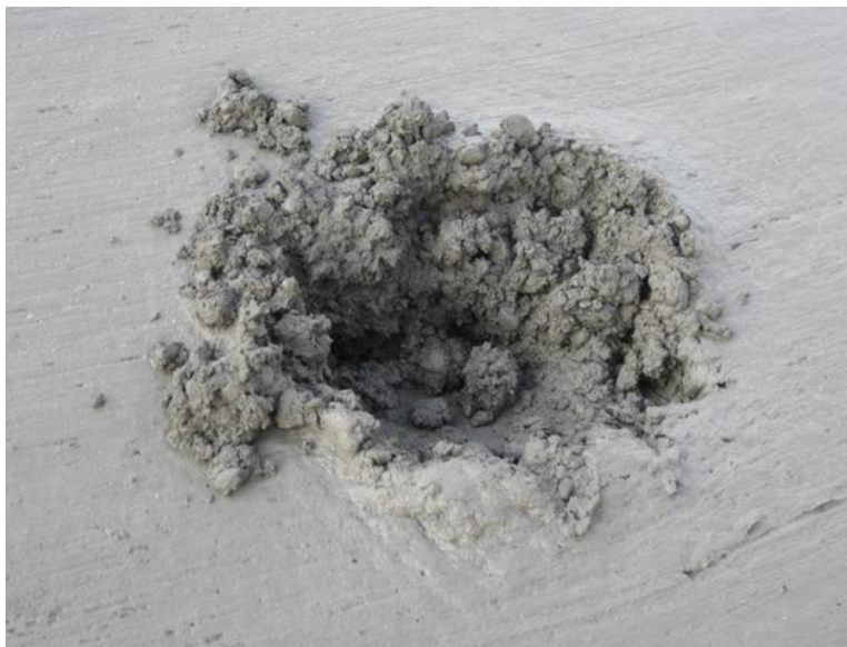
Figure 19. Concrete surface after a sample has been removed from behind the paver
