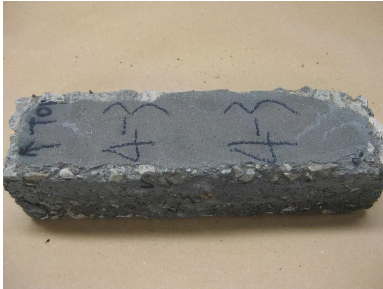
Figure 14. Damage in a beam after an ASTM C 666 test
