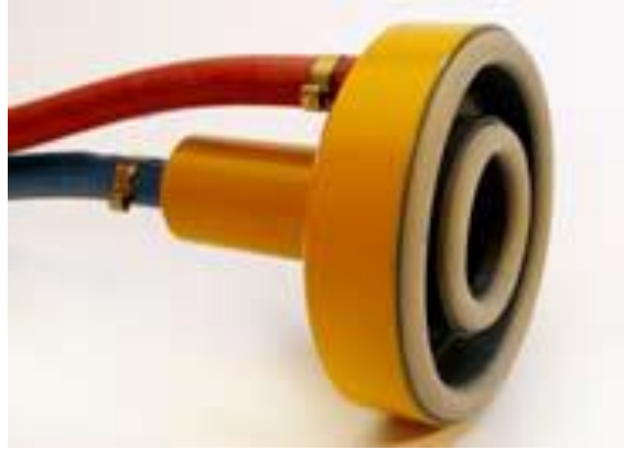
Figure 12. Torrent test cell (Proceq)
