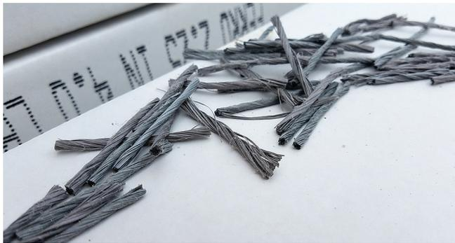
Figure 25. Synthetic fibers
