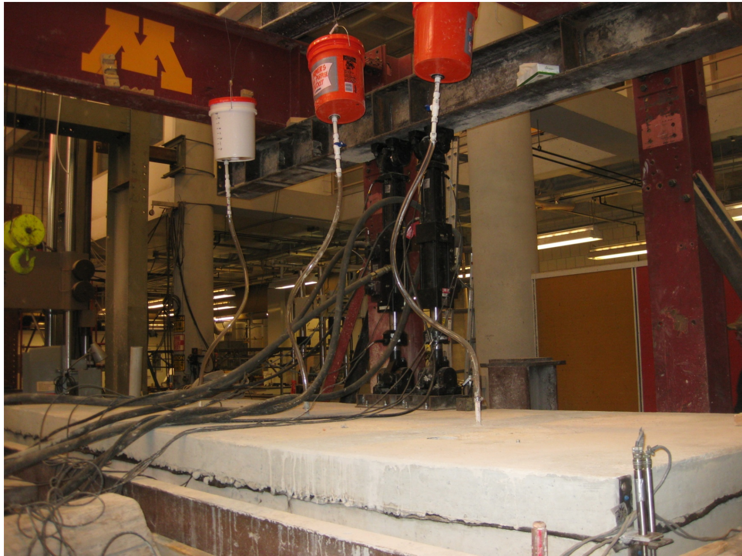
Drainage experiment set-up
