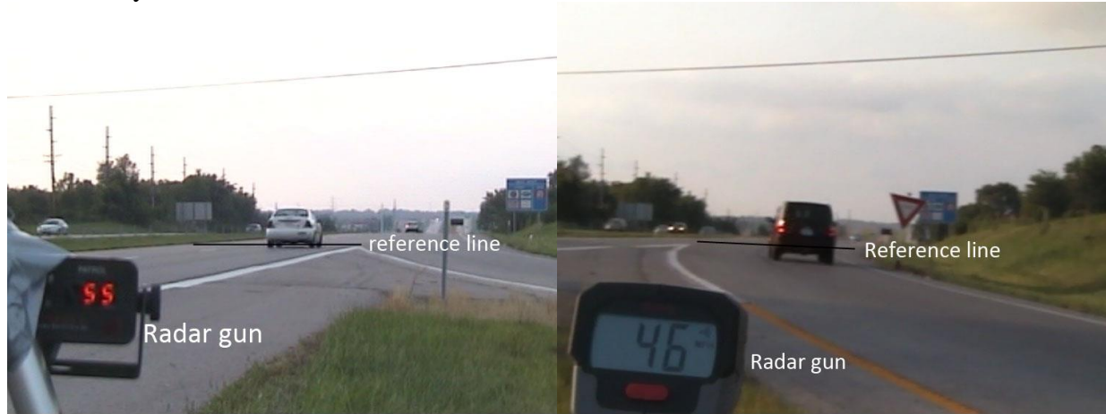
Figure 3.2 Mainline camera vision (left) and Ramp camera vision (right).
