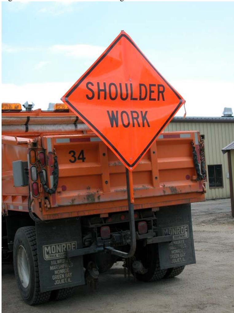
Figure 4. Rollup Sign and Holder on Rear of a Truck
