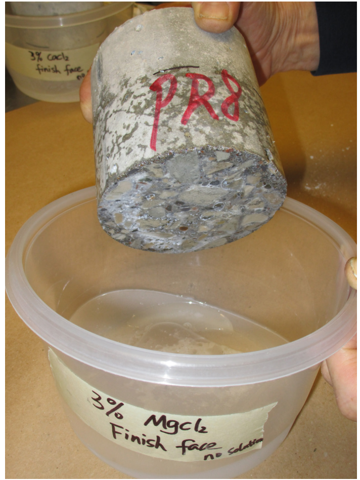
Figure 4: A cylinder that had been soaked in MgCl_2 solution then exposed to air for 6 months. Note that it still appears wet – demonstrating the effect of MgCl_2 in increasing saturation.
