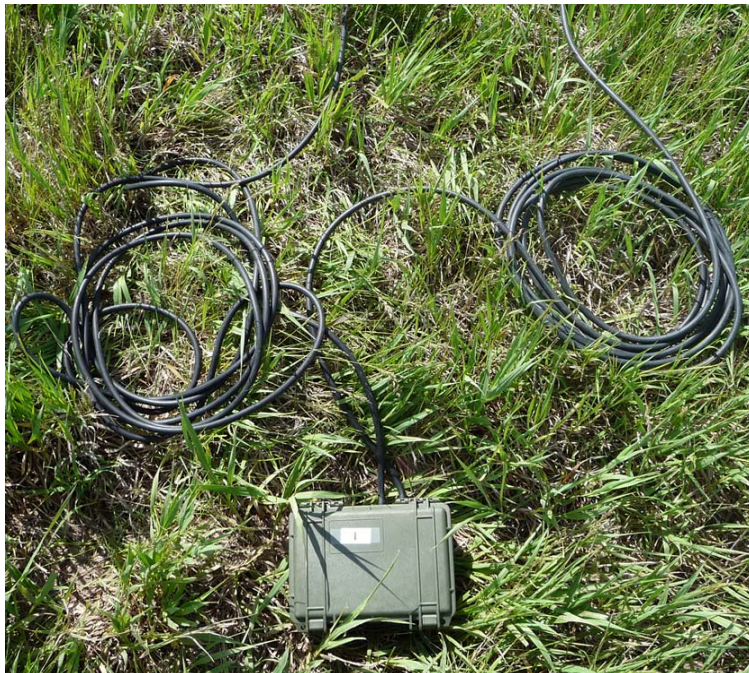
Figure 4.8 A Speed Sensor Connected with Road Tubes
