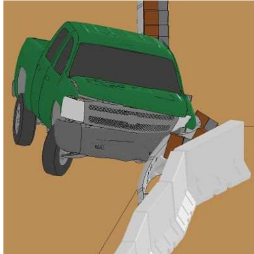
Figure 58. Bowing of Thrie Beam at Impact Location No. 7
