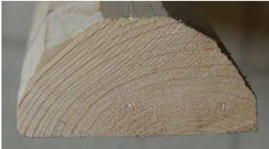
Figure 27. Cross-section of a 1.50"-radius prototype.
