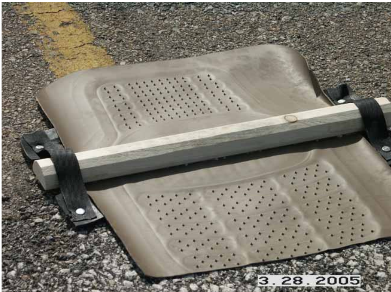
Figure 29. Wooden prototype rumble strip in place for testing.
