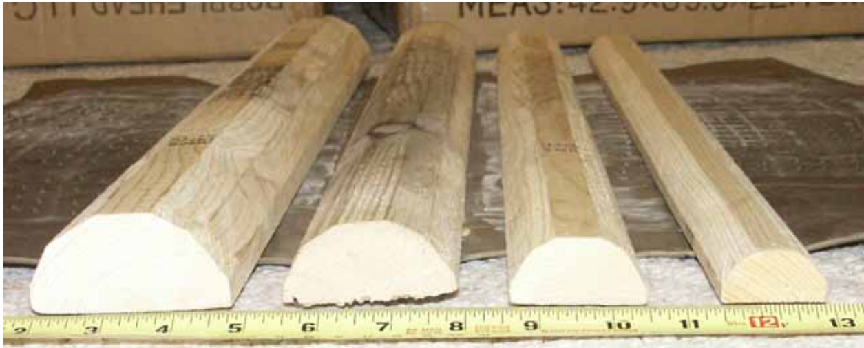
Figure 28. Section view of four sizes of prototype rumble strips, 1.50'' to 0.75'' (L to R).
