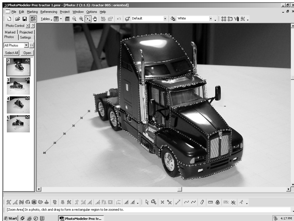
Figure 7. Marking cab features on photograph
