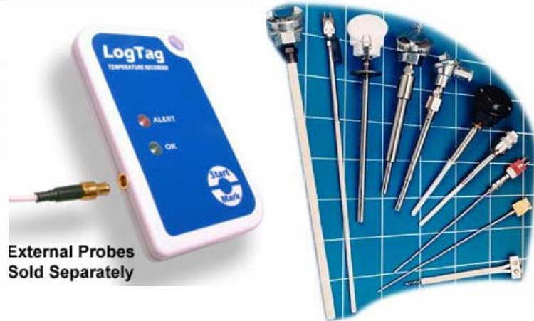
Tipped Probe (Available in 1.5 meter and 3.0 meter cable length) A tipped 150mm length 5mm OD 316 stainless probe with no handle. Probe and Cable are FDA food rated. Each probe comes with a 1.5 Meter or 3.0 Meter length cable terminated with an MCX plug for input into the LogTag TREX Recorder.
