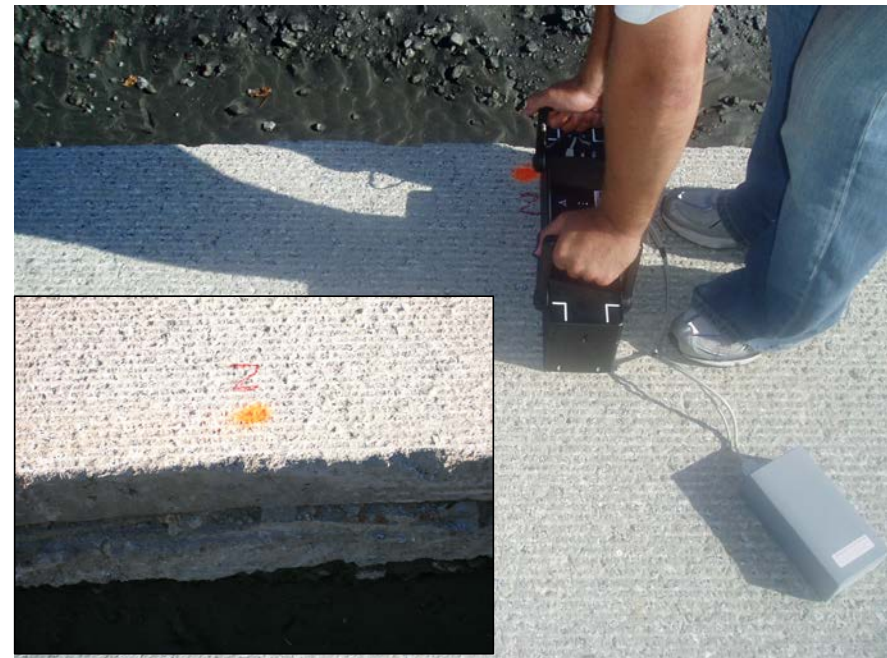
Ultra-Sonic Testing Device: MIRA
