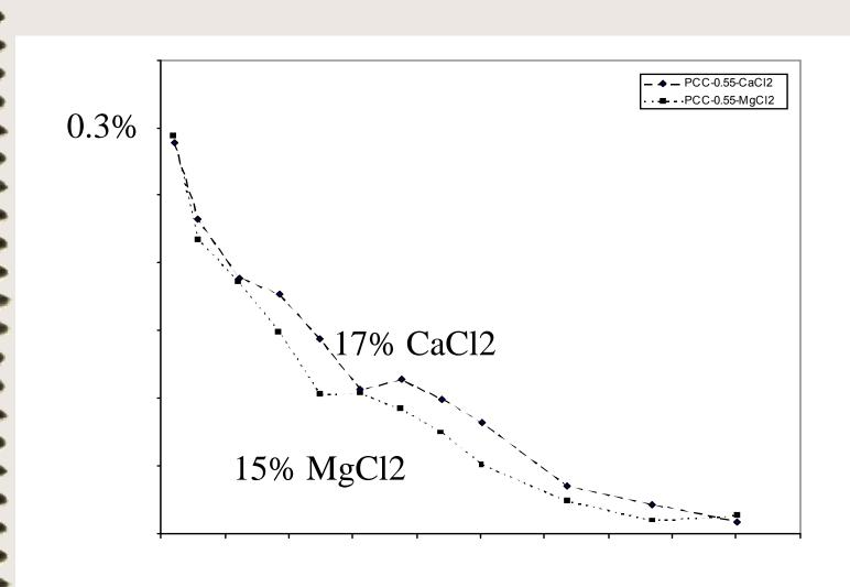
Typical Diffusion Profiles for 0.45 *w/c* Concrete Exposed to 15% MgCl<sub>2</sub> - PCC, 15% Fly Ash, 35% GGBFS Mixtures
