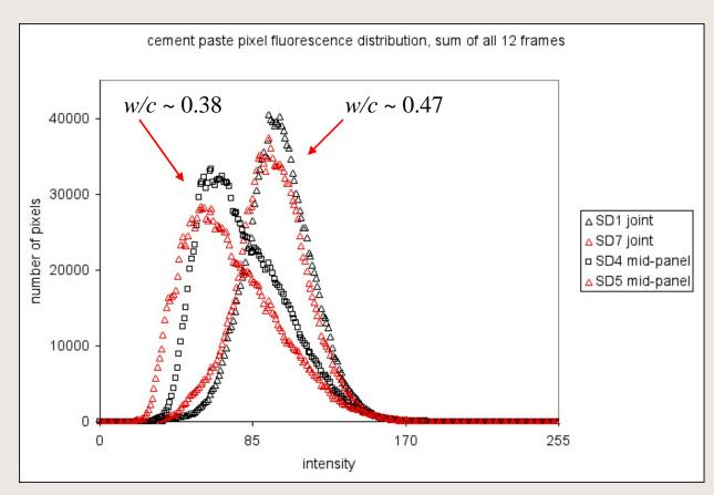
• Histogram comparing cement paste pixel intensities using all 12 frames as collected from thin sections prepared from cores taken at the joint versus cores taken mid-panel.
