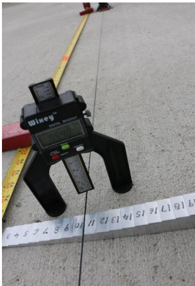
Figure 17. Digital height gauge used for measurements
