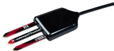
Figure 11. Decagon 5TE sensor for measuring relative dielectric permittivity, electrical resistivity, and temperature
