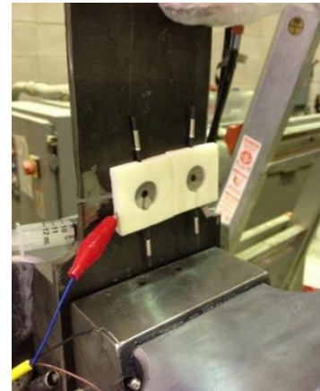
(b) Sensors installed at the crack location
