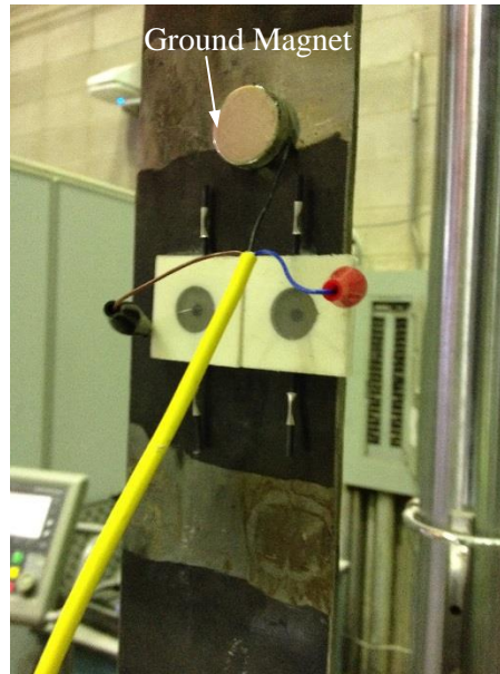
(b) View of Ground Magnet and Sensors on Specimen
