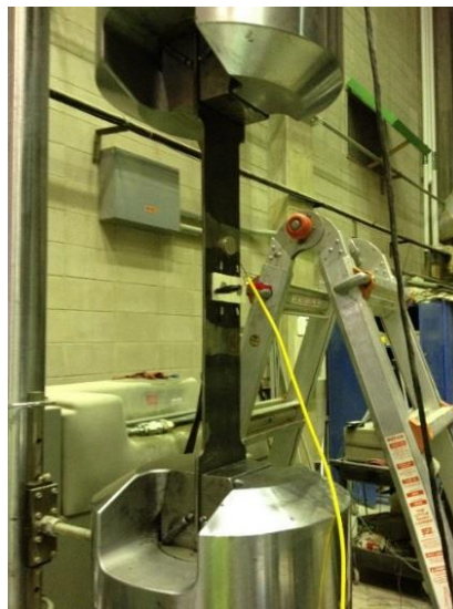
Figure 5. Fatigue load test setup
